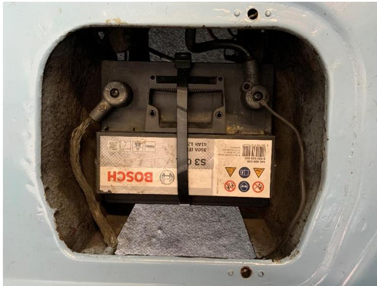
Two other alternatives are the B036 and more commonly available type 202. Both batteries are the same size as a single 6V battery and can be fitted and secured using the existing battery clamp.
