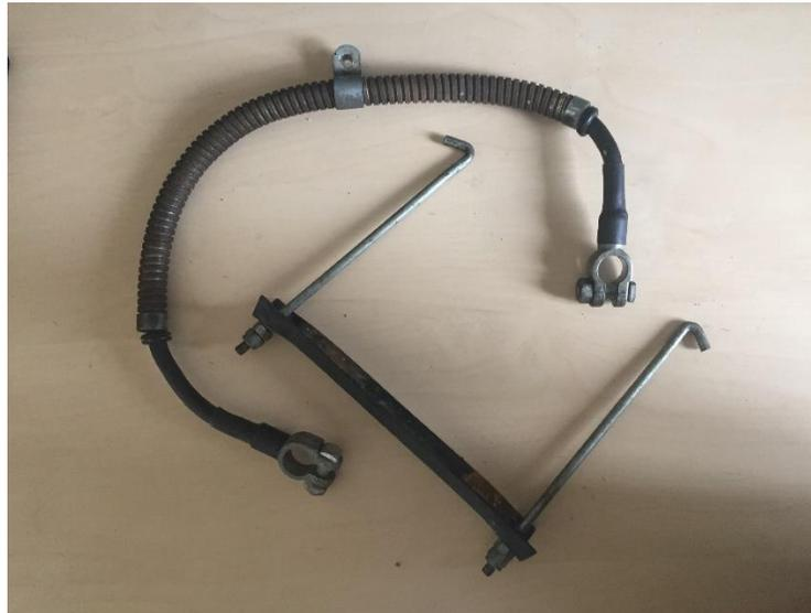
7. Unbolt and remove the earth lead from the left hand battery compartment. This will need to be relocated to the right hand battery compartment.
