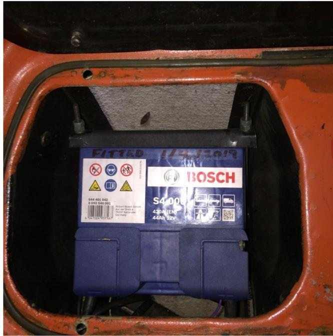
13. Secure the battery cover back in place with the 5 x Zeus fasteners , refit the carpet/ seat cover
